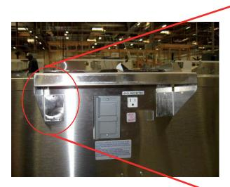
2.- Drill holes and screw in place (with screws provided – Hex Tek S/S 10-16 X ½")
